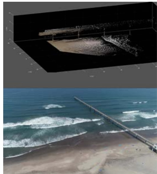
LiDARを用いた波・地形の連続観測と海底地形測量のための UAV を用いた海面動画撮影 Continuous measurement of waves and topography change using a LiDAR scanner, and video shooting using a UAV for nearshore depth estimation.
