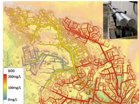
管路内実験装置 (右上) と管路内浄化のシミュレーション An experimental unit of in-sewer purification pipe (right-top) and water quality simulation of in-sewer purification
