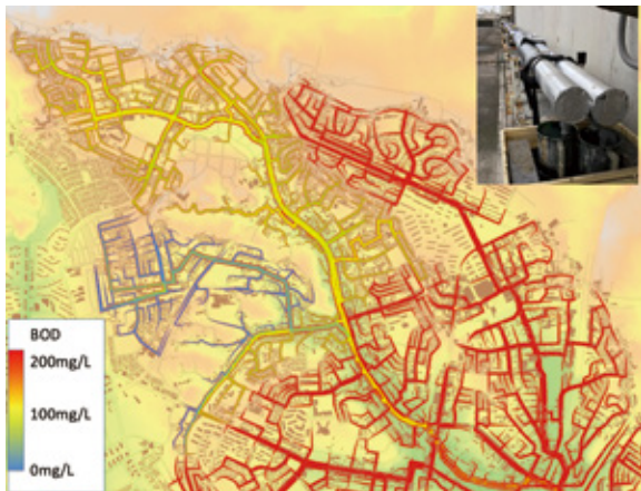
管路内実験装置（右上）と管路内浄化のシミュレーション An experimental unit of in-sewer purification pipe (right-top) and water quality simulation of in-sewer purification
